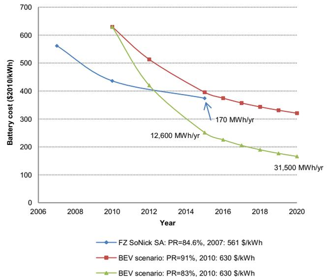
**Fig. 4.** ZEBRA battery cost scenarios, based on cost data from Kalhammer et al. [8]. Blue line: based on production capacity goals of FZ SoNick [76]; red and green line: based on cumulative production volume of 7.1 million batteries in 2020. Annual production capacities in 2015 and 2020 are given for FZ SoNick and BEV scenarios. (For interpretation of the references to color in this figure legend, the reader is referred to the web version of this article.)
