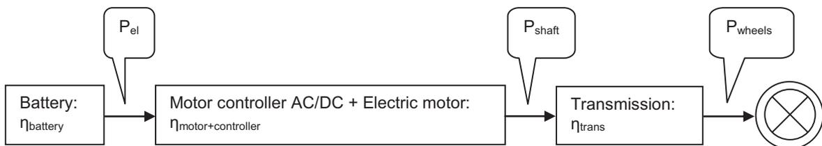
Fig. 1. Main elements and power flow inside a battery electric vehicle, adapted from Campanari et al. [3].
