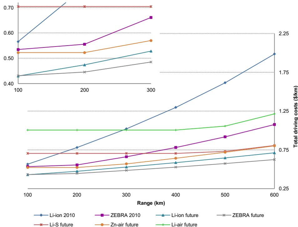
Fig. 10. Total driving costs of the battery electric car, considering a number of present and future battery technologies (at an electricity price of 0.110 \$ kWh<sup>-1</sup>, including VAT [4,96]).
